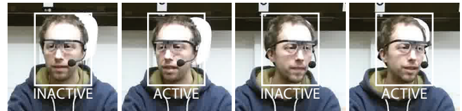
Fig. 1. Example of a vision-based voice activity detector. The first and second images capture negative head rotations around the Y-axis (yaw) w.r.t. the camera origin, while the third and fourth images represent positive rotations.
